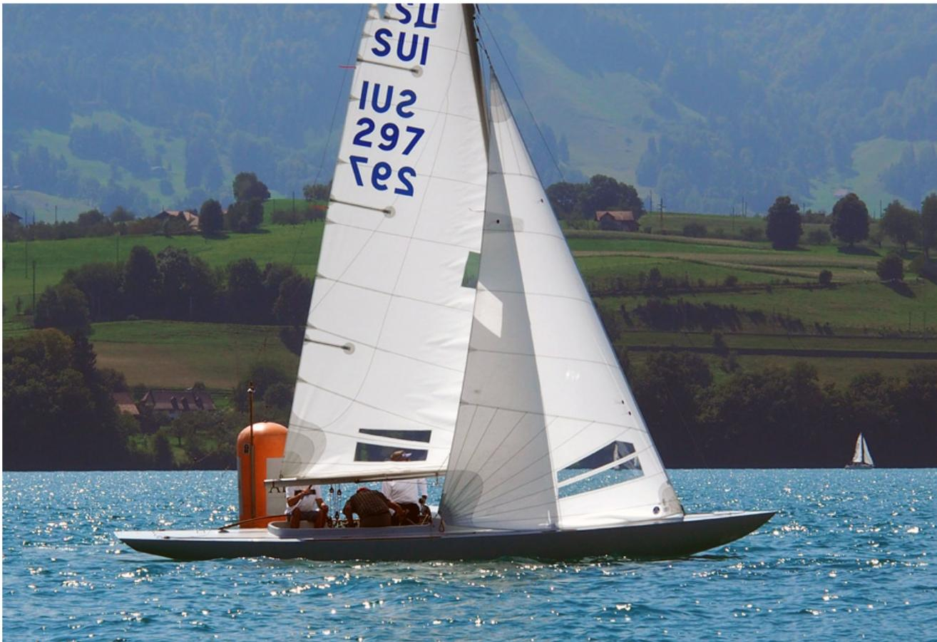
Tuning a Dragon starts with measuring forestay length and includes other complexities such as running backstays and adjustable shrouds that can be tensioned underway. Photo: North Sails Schweiz
